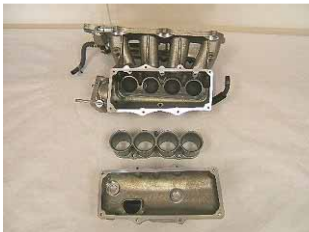
Inside of Intake manifold
